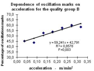
Figure 4: Oscillation marks and acceleration
