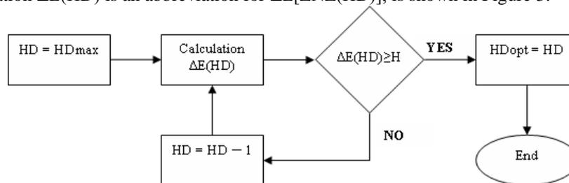
Figure 3 The flowchart of the optimization algorithm idea
